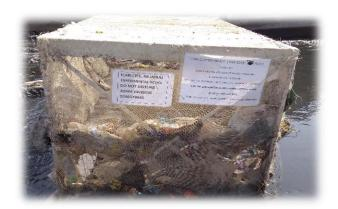
Microplastic, macro- and megaplastic collected in the lower compartment of the device during post-high tide duration. The upper compartment shows the plastic and floating debris collected during high tide
